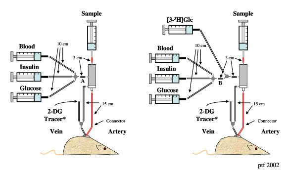
Figure 1. Scheme illustrating the connection of catheters, dual channel swivel, and infusates in relation to the mouse when clamping without (left panel) or with (right panel)  $[3-{}^{3}H]$ glucose. Diagram is not to scale. \*This port is generally for 2-deoxyglucsoe (2DG) tracer bolus administration, but can be used for other infusates as well. A and B indicate the 3 cm microrenathane tubing filled with non-heparinized saline and capped with a stainless steel plug (see step 6).
