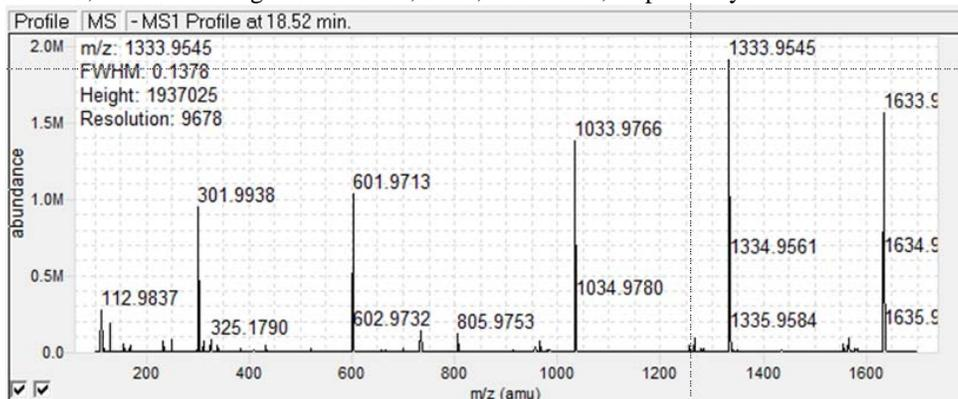
e. If the intensity of even one of the selected ion is below this value clean the ion source and repeat the instrument tuning.
