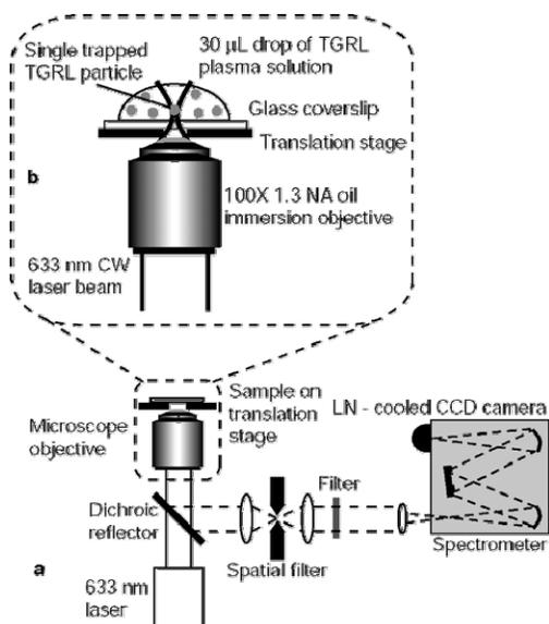
**Figure 2. (a) Confocal spectroscopy system for the detection of the Raman spectra of single lipoprotein particles. (b) Optical trapping of a single lipoprotein particle in plasma solution or cell and simultaneous spectral acquisition using a single laser beam focused through a high numerical aperture objective.**
